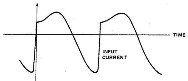
Figure 2. Distorted Forward Current in Step Recovery Diodes
