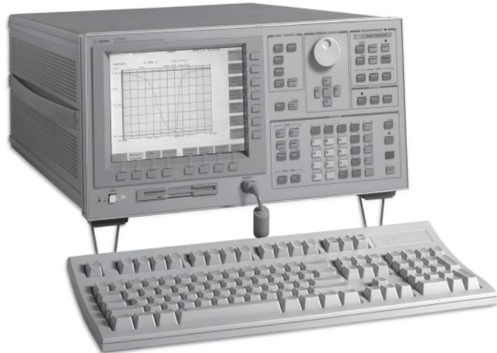
Figure 3. Agilent 4156C Precision Semiconductor Analyzer
