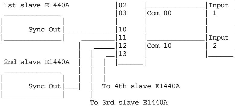
Try to keep the Sync Out path lengths as equal as possible. The same applies to the main outputs. Perform a phase measurement at the device and note any offset needed. With propagation times equalized, the phase accuracy lies in the range /-1 to /- 7 degree depending on waveform and amplitude mix, and frequency.
