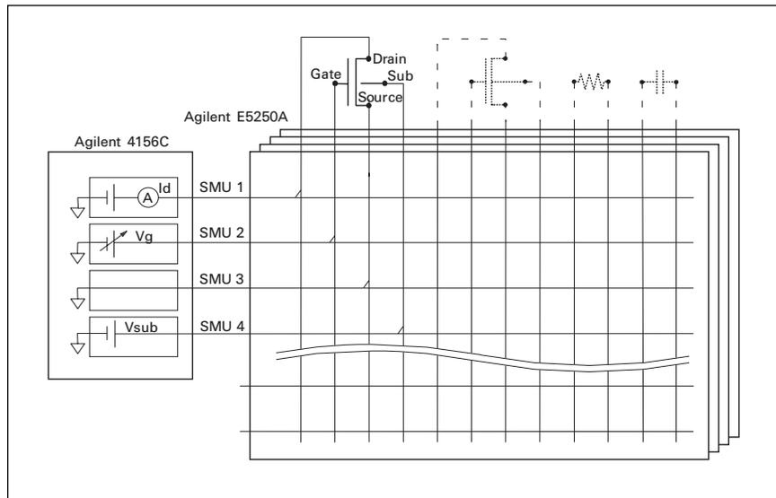
**Figure 3. Measurement diagram of the Id-Vg curve of n-channel MOSFET**
