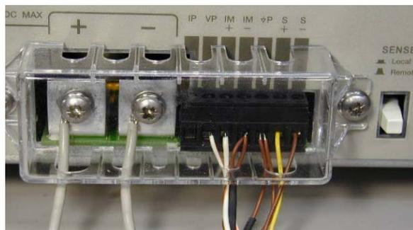
Figure 8. Power supply terminal connection
