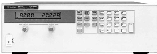
Figure 1. Agilent 665xA series Performance DC Power Supply
