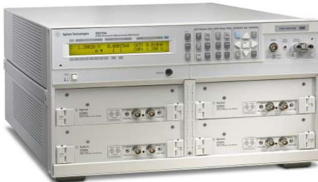
Agilent E5270A 8 Slot Parametric measurement Mainframe with 4 SMU plug-in modules
