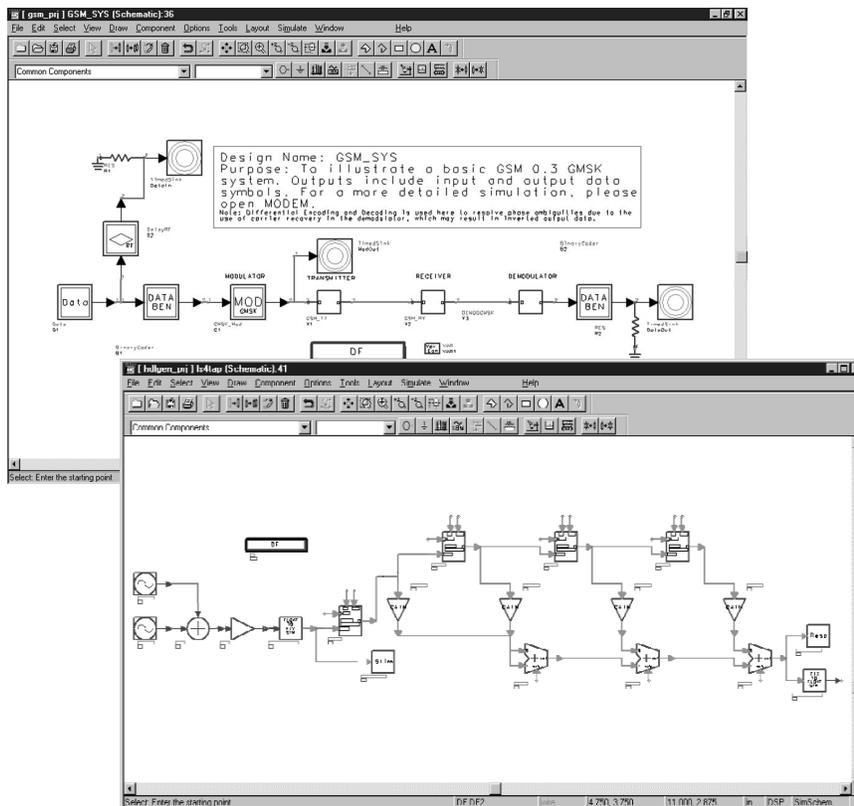
When the system-level design is complete, the synthesizable models allow you to generate HDL code efficiently.
