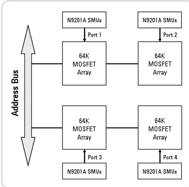
Figure 15. The Array-C architecture supports the measurement of multiple arrays on the wafer simultaneously using a multi-site probe card.
