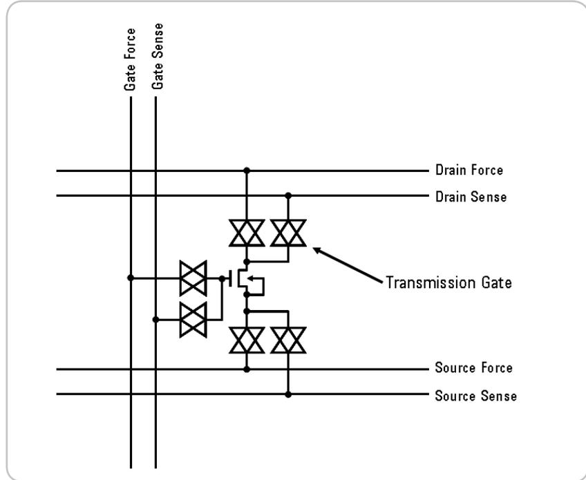
Figure 6. Typical arrangement to perform a Kelvin measurement on a MOSFET device in an addressable array.
