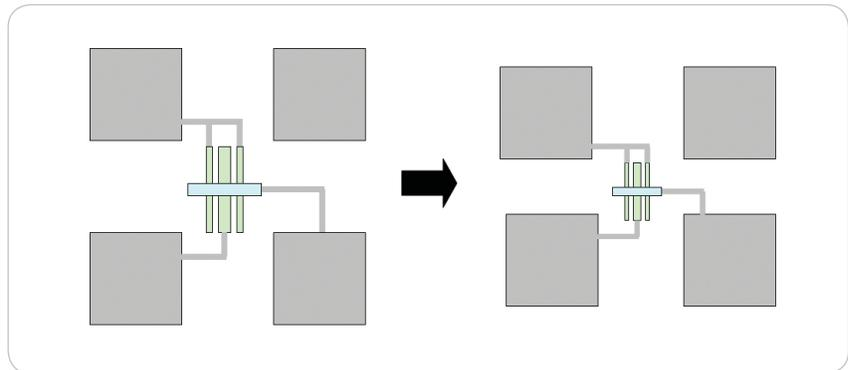
Figure 2. Probe pads cannot scale with process design rule and scribe line scaling, which limits the number of devices that can be placed into the scribe line using conventional test structure arrangements.
