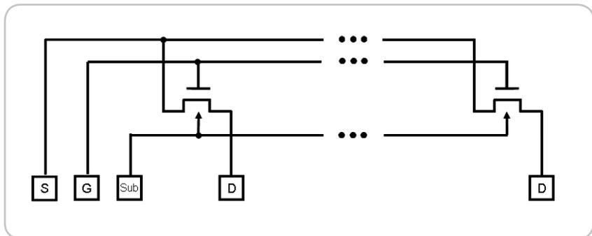
Figure 4. Passive array test structure organization.
