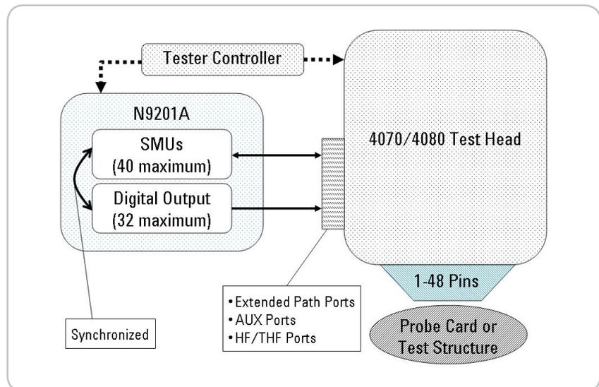
Figure 8. The N9201A option can supply up to 32 digital outputs and 40 SMUs, and it makes sure that the addresses are synchronized with the SMU measurements.
