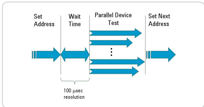
Figure 9. The N9201A option synchronizes the address outputs with the parallel measurements performed by the SMUs. The wait time between address set and measurement is programmable with 100 μs resolution.
