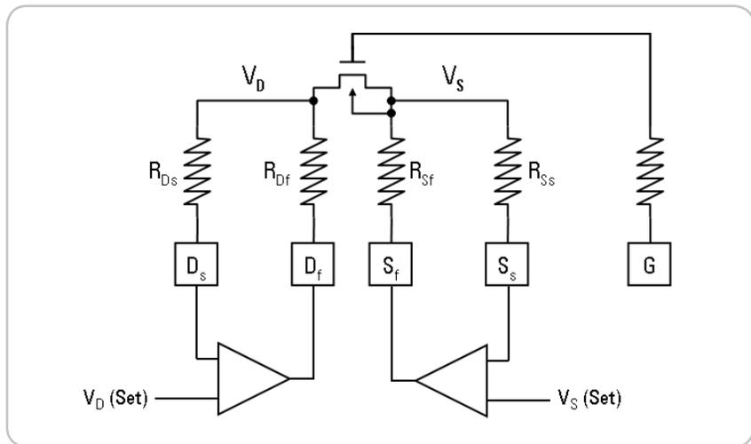
Figure 17. Kelvin SMU Method – The force and sense inputs of the Kelvin SMU can be connected directly to the force and sense pads (respectively) of the addressable array to remove the effects of series resistance in the lines.
