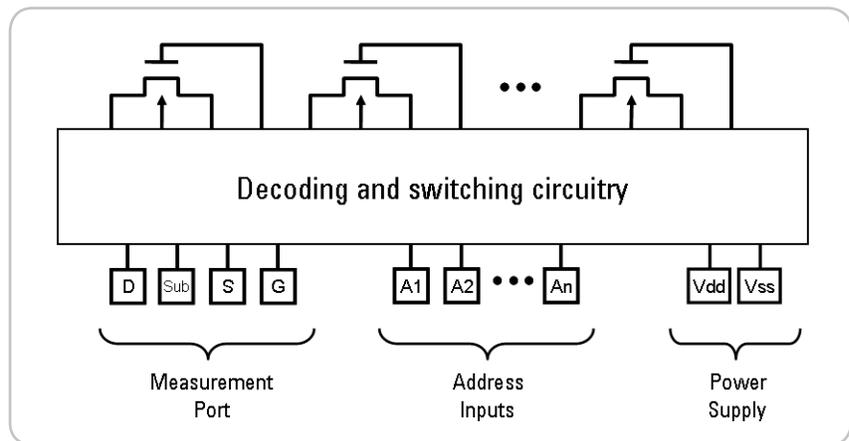
Figure 5. Addressable array example.
