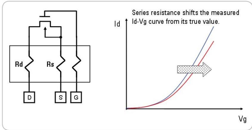
Figure 16. The series resistance in the signal lines going to the MOSFET distorts the actual voltage applied to the DUT.
