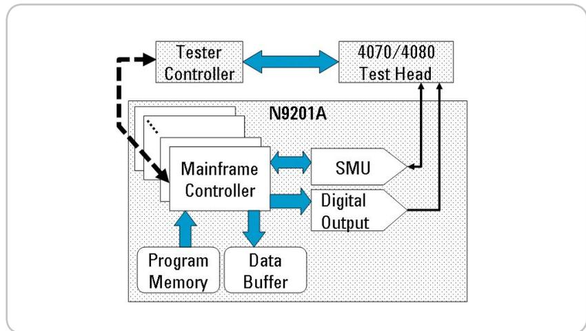
**Figure 10. The N9201A option has TIS commands that allow you to load the program memory of the SMU mainframes. Combining program memory with parallel test yields better throughput than that obtainable using parallel test alone.**
