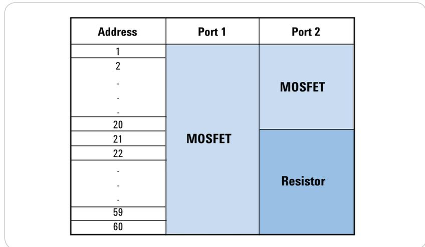
Figure 11. Array-A has two measurement ports that connect to 60 devices each.
