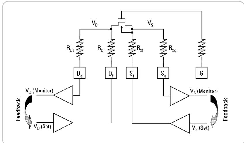
Figure 18. Monitor and Adjust Method – In this method a separate measurement resource is used (SMU or VMU) to monitor the actual DUT voltage and the applied voltage is adjusted until the voltage at the DUT equals the desired value.
