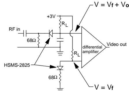
Figure 1: DC differential detector
