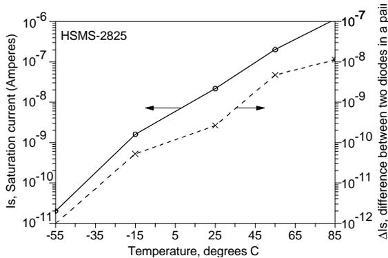
Figure 4:  $I_s$  and  $\Delta I_s$  vs. temperature
