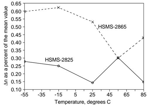
Figure 6:  $\Delta n$  vs. temperature, two diode types
