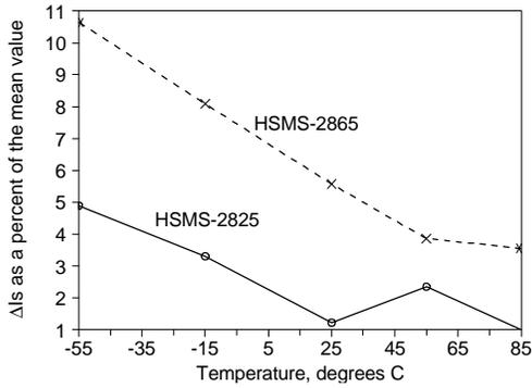
Figure 7:  $\Delta I_s$  vs. temperature, two diode types
