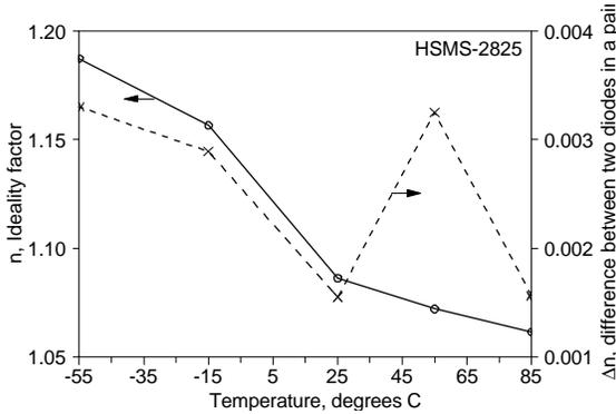
Figure 3:  $n$  and  $\Delta n$  vs. temperature
