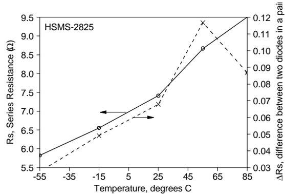
Figure 5:  $R_s$  and  $\Delta R_s$  vs. temperature
