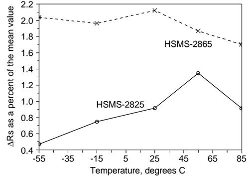
Figure 8:  $\Delta R_s$  vs. temperature, two diode types
