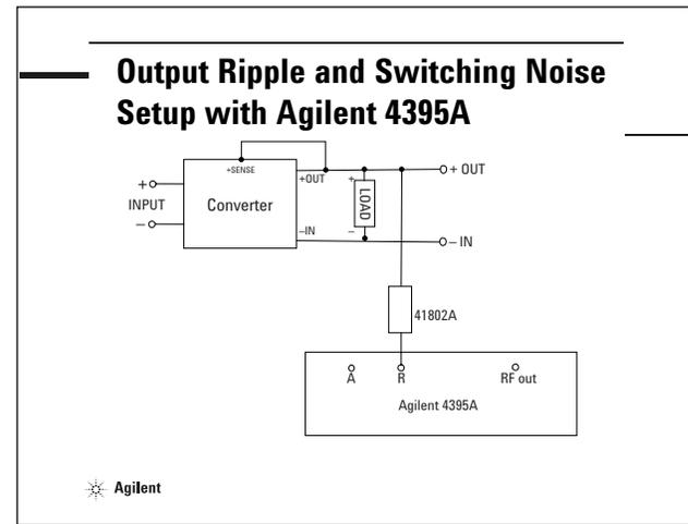
This figure shows the equipment setup for output ripple and switching noise measurement with the Agilent 4395A. The spectrum analyzer measures at the output terminal (+OUT) of the switching power supply with the Agilent 41802A.
