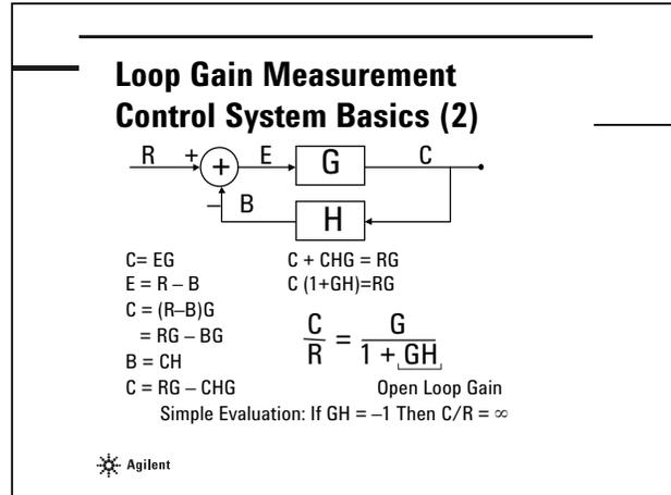
The simple feedback control system model is shown again in this figure. From this simple model we can derive the input/output relationship of a closed-loop system as  $C/R = G/G(1 + GH)$ . This expression is known as the closed-loop transfer function. GH is the open-loop gain function. A simple evaluation of this equation shows that:
