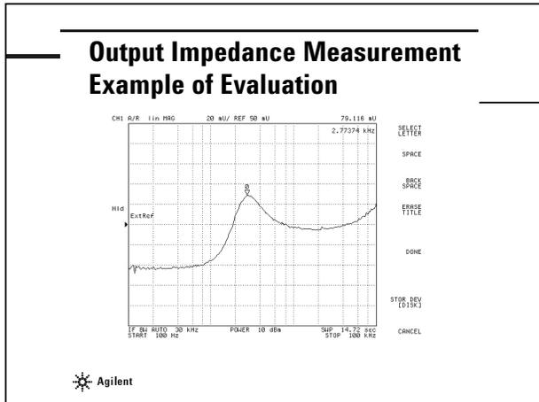
This figure shows an example of the output impedance measurement with the 4395A.
