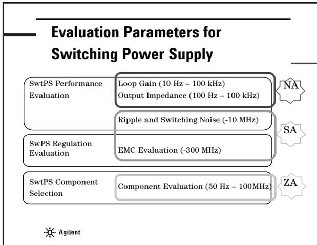
Designers evaluate the switching power supply for various reasons, such as for performance evaluation, regulation evaluation, and components selection. The summary of the evaluation parameters for switching power supply are shown in this figure. As you can see from this figure, the designers need three different analyzers; network, spectrum, and impedance analyzers with the frequency range from 10 Hz to 300 MHz.
