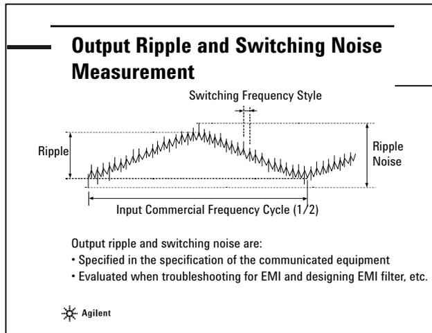
The wave of a ripple noise is described in this figure. The ripple consists of the frequency that is twice as large as the power line frequency, the switching frequency, and other irregular ripples. They appear at the output of the switching power supply. The ripple noise is expressed in peak-to-peak volts in the specifications of the switching power supply. The spectral characteristics of power supplies used in communication equipment are frequently specified.
