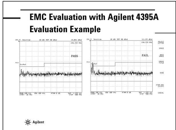
This figure shows an example of the EMC evaluation with the limit line function of the 4395A.
