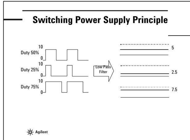
This figure illustrates the switching behavior. The pulse width modulator generates the pulse where duty rate is changed according to the output of the error amplifier. The right-hand side of this figure shows the output of the pulse width generator, and the left-hand side of this figure shows the output voltage from the low pass filter. You can see that the output level of the voltage is changed by the duty rate of the pulse.
