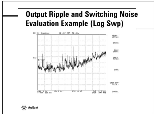
This is an evaluation example of the output ripple and switching noise measurement with log sweep. You can see a lot of spectrums generated from the switching frequency and its harmonics. The 4395A does not have the log sweep mode, but it can be executed with the list sweep mode and an IBASIC program.
