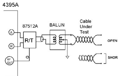
During the attenuation measurement a grounded shield should be used to isolate the two ends of the cable.
