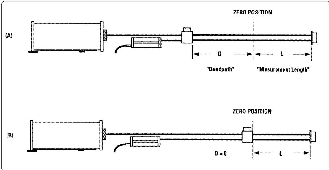
Figure 8. Optical configuration with and without deadpath.
