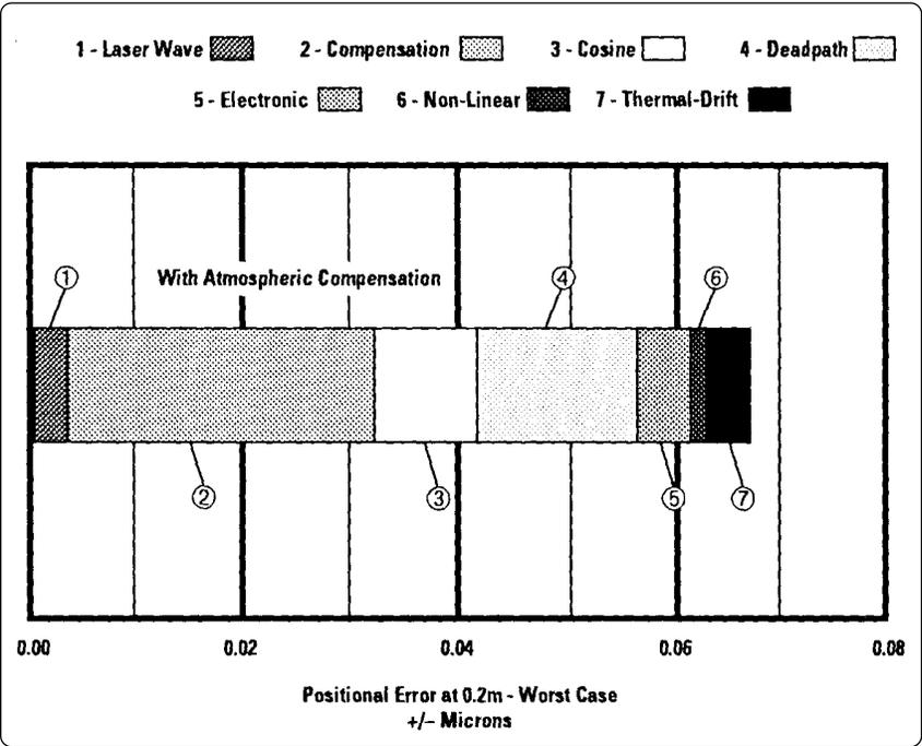
Figure 20. Worst case system accuracy with atmospheric compensation for the wafer stepper example.
