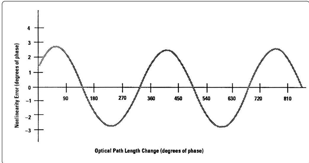
Figure 3. Worst-case error resulting from imperfect separation of the two beam components.
