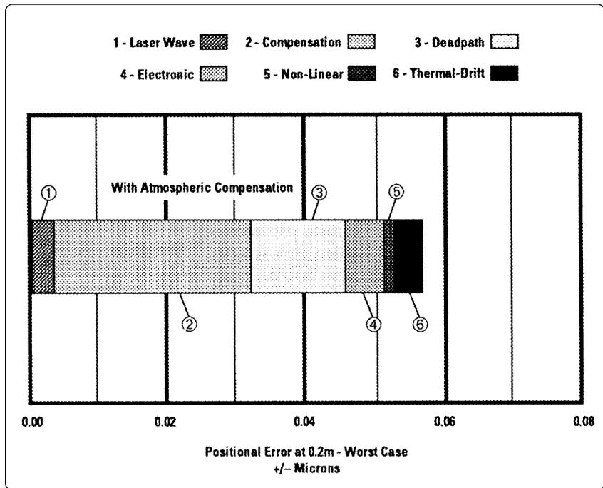
Figure 22. Worst case system long-term repeatability with atmospheric compensation for the wafer stepper example.
