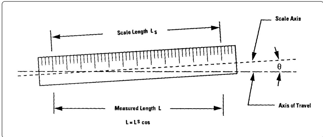
**Figure 10. Scale misalignment causing cosine error.**
