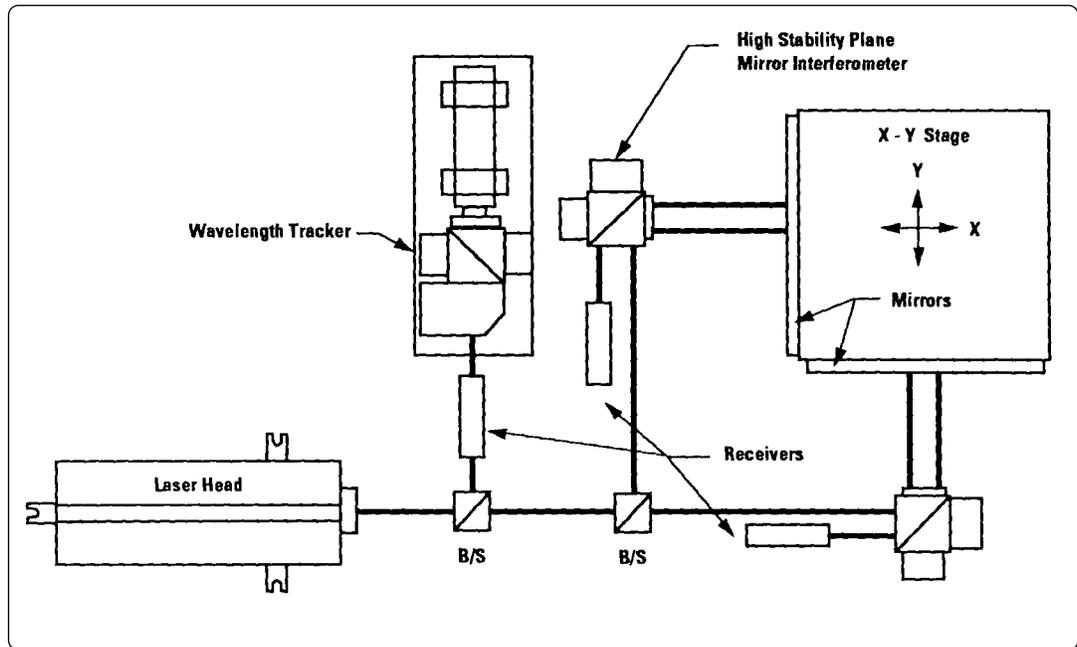
Figure 18. Laser system configuration for an I.C. wafer stepper.
