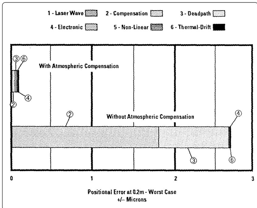
Figure 21. Worst case system long-term repeatability with and without atmospheric compensation for the wafer stepper example.
