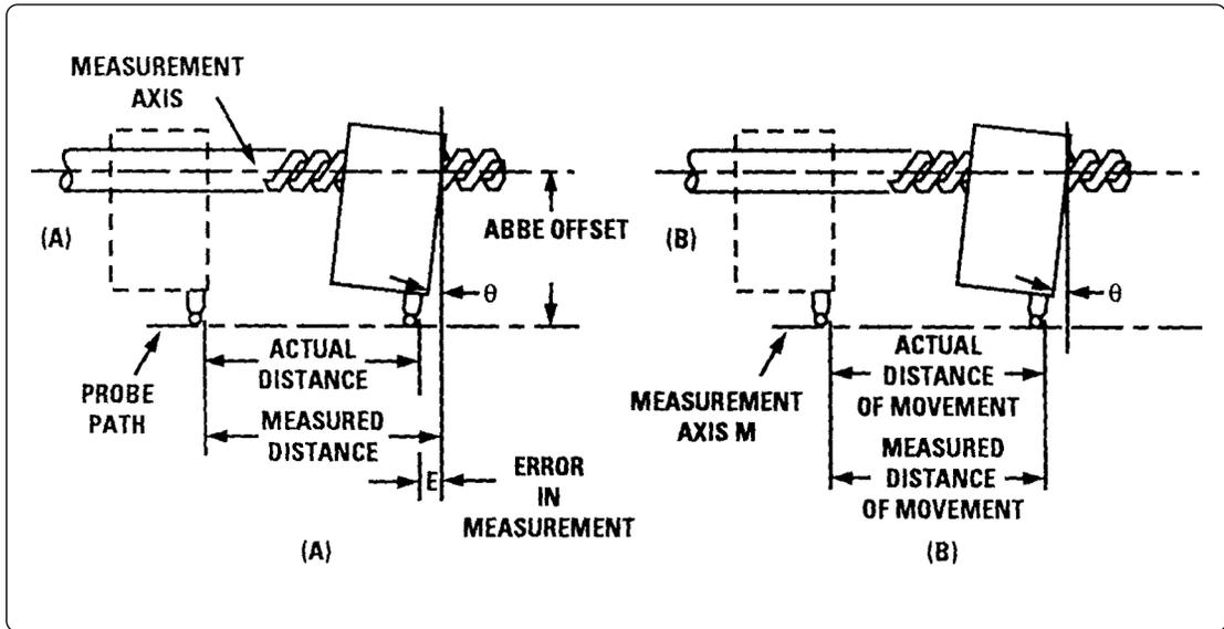
Figure 9. Illustration of Abbe' error.
