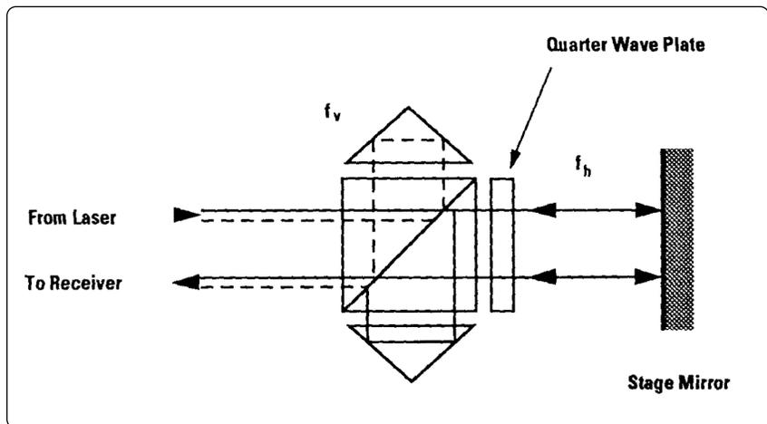
Figure 4. Conventional plane mirror interferometer with unequal path lengths that result in optics thermal drift.
