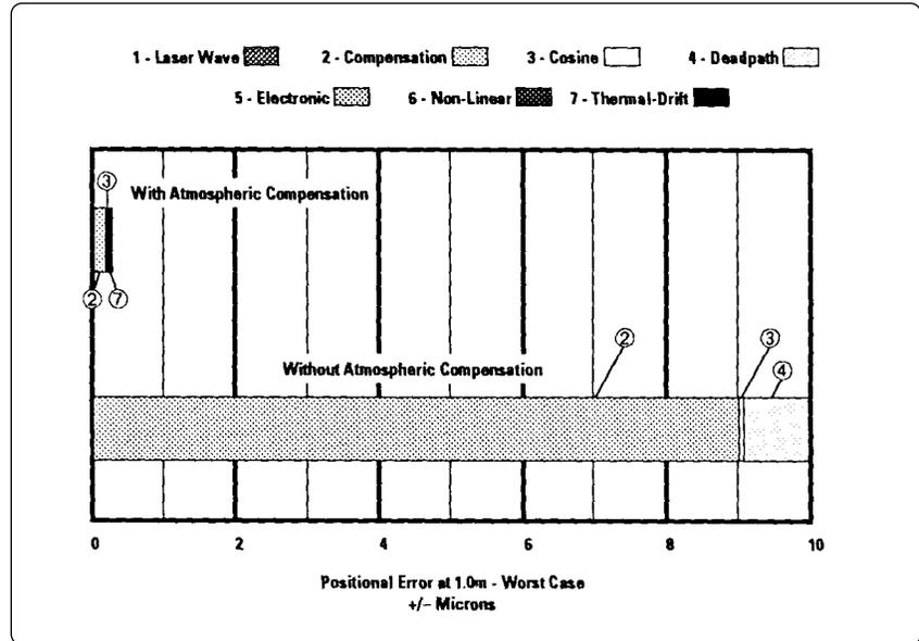
Figure 14. Worst case system accuracy with and without atmospheric compensation for the CMM example.
