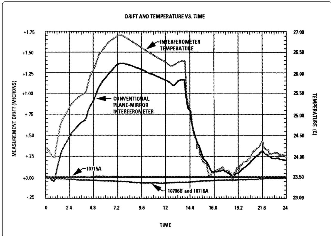
Figure 6. Optics thermal drift comparison between different interferometers.
