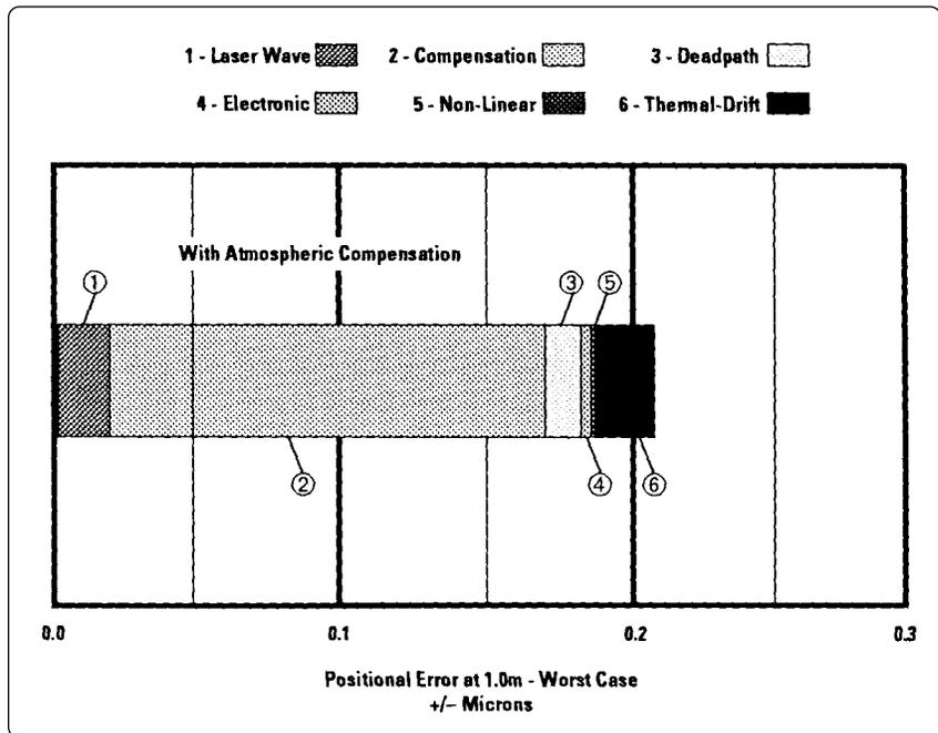
Figure 17. Worst case system repeatability with atmospheric compensation for the CMM example.
