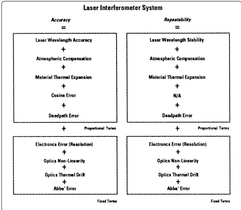
Figure 11. Laser Interferometer System Accuracy and Repeatability Error Budgets.
