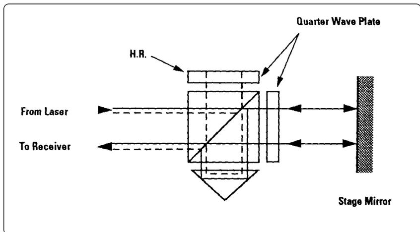
Figure 5. Optical schematic for the Agilent 10706B High stability plane mirror interferometer. Equal beam paths in the interferometer significantly reduce the optics thermal drift.
