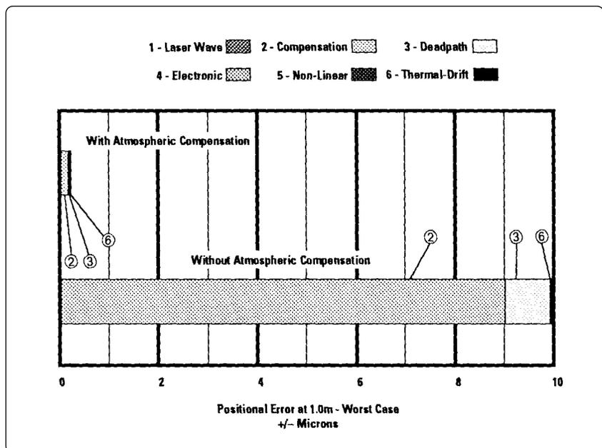
Figure 16. Worst case system repeatability with and without atmospheric compensation for the CMM example.
