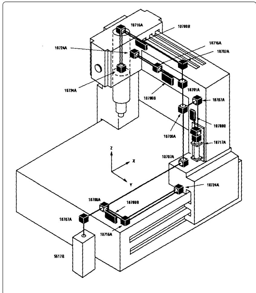
Figure 13. Laser system configuration for a precision CMM.
