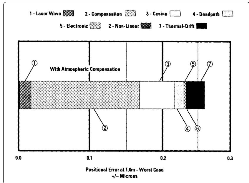
Figure 15. Worst case system accuracy with atmospheric compensation for the CMM example.
