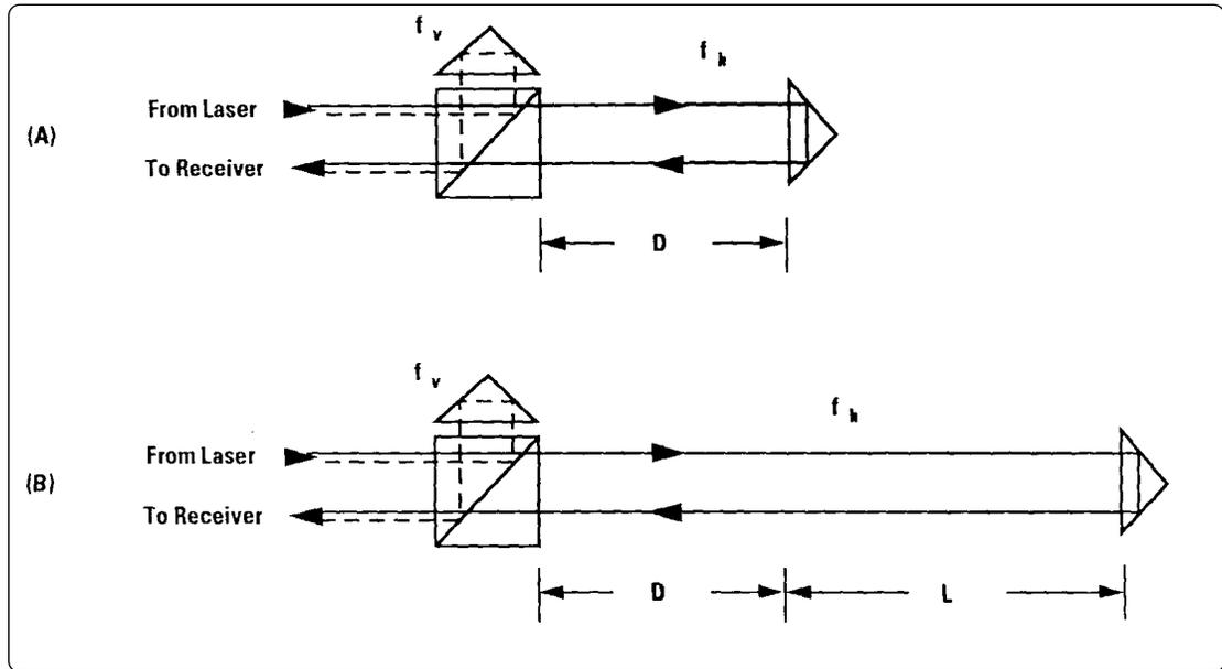
Figure 7. Deadpath caused by unequal lengths from initial point.
