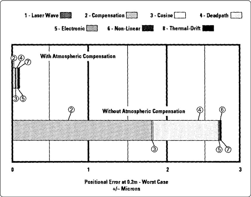
Figure 19. Worst case system accuracy with and without atmospheric compensation for the wafer stepper example.
