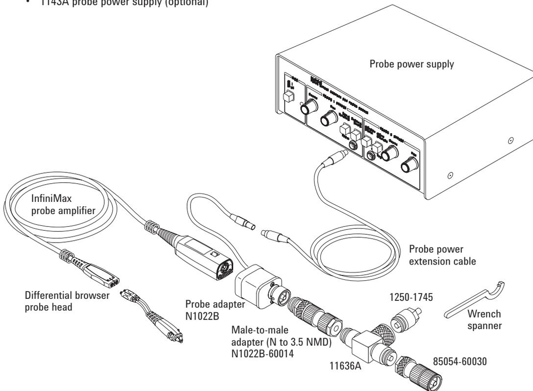
Adapting and splitting signals for probing and clock extraction with the 83496A/B option 101
