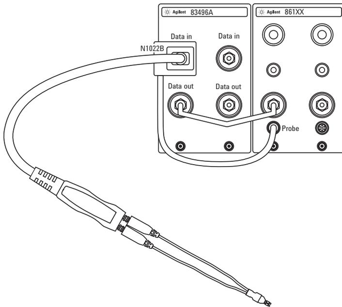
Figure 4: Connector scheme using the 83496A/B and N1022B
