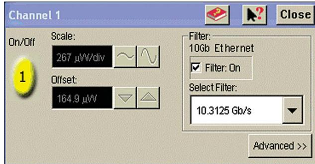
Figure 7: Reference receiver filter setting
