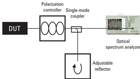
Figure 22: Optical spectrum analyzer setup
