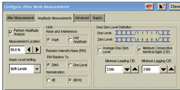
Figure 10: Amplitude measurement configuration
