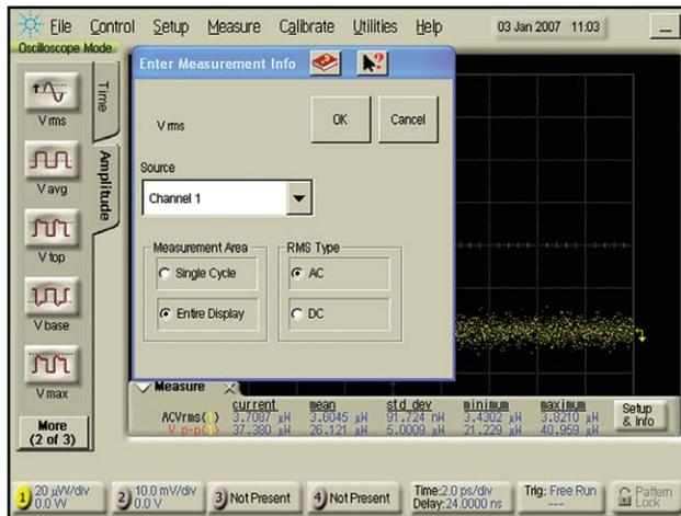
**Figure 15: Intrinsic noise measurement: N<sub>opt(dark)</sub> = 3.7μW**
