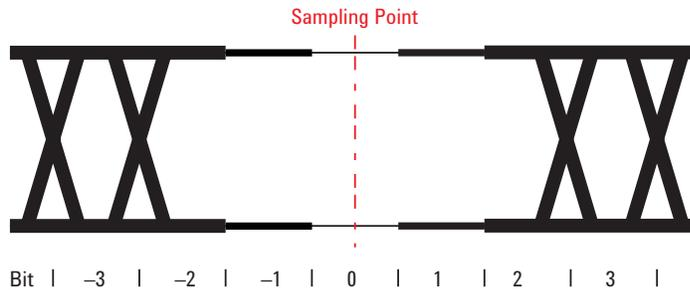
Figure 5: Sample point to measure random amplitude variations
