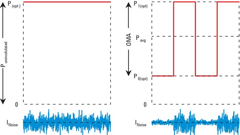
**Figure 2: Conceptual difference between RIN (left) and RIN OMA (right)
