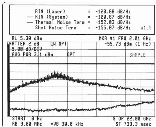
Figure 19: RIN spectrum of a Fabry-Perot laser (fluctuations in the modal distribution contribute to additional intensity noise)
