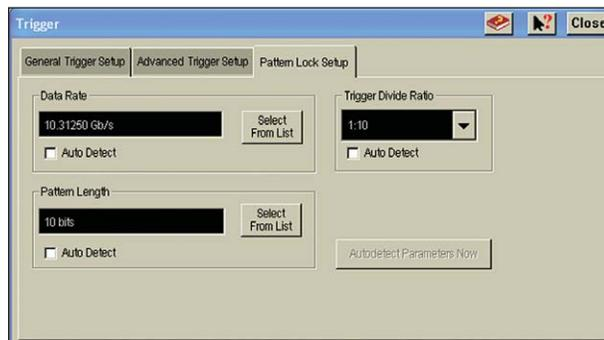
Figure 13: Pattern lock setup for square-wave modulation (pulse generator: 1.03125 GHz square wave simulating a 0000011111 pattern at 10.3125 Gb/s)
