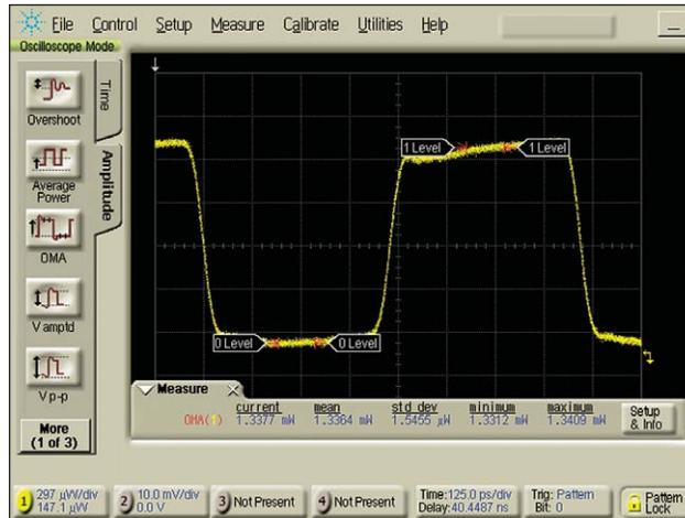
Figure 3: OMA measurement on a square-wave signal
