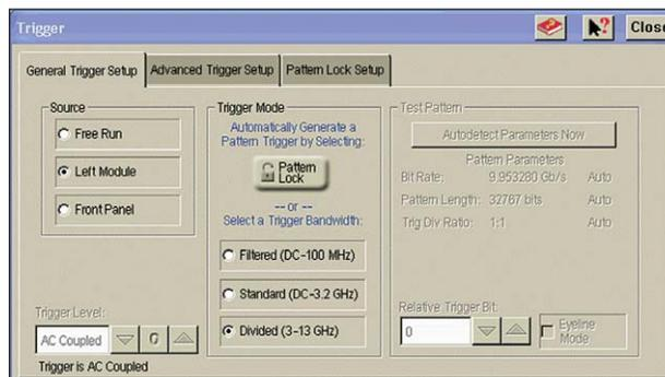
Figure 6: Trigger setup for trigger signals > 3.2 GHz<sup>4</sup>
