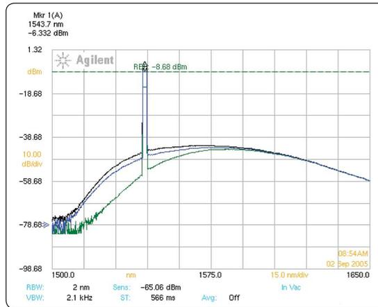
Figure 27: EML spectra ("1" level, average power and "0" level)
