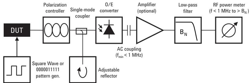
Figure 16: IEEE 802.3ae based setup for RIN OMA
