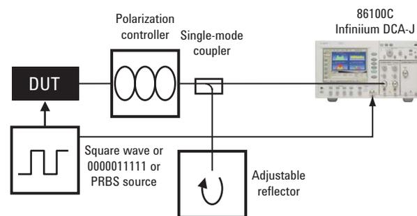
Figure 4: Agilent 86100C Infiniium DCA-J based setup<sup>3</sup>
