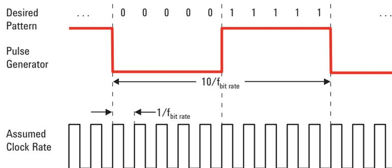
Figure 12: Square wave from pulse generator simulating 0000011111 pattern
