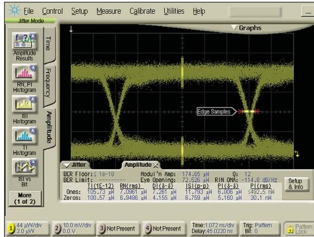
Figure 11: RIN OMA result (normalized to 1 Hz)
