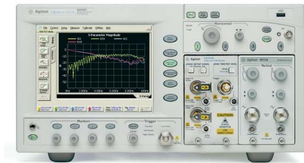
Tests SI-01 through SI-08 use Time Domain Reflectometry (TDR) techniques to measure impedance in the time domain with test results reported in the time domain or frequency domain (S-Parameters) as required by the standard. The 86100C DCA-J with option 202 can easily translate between the time and frequency domains with a single button push.
