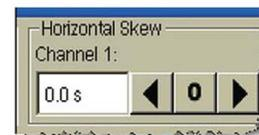
Horizontal skew adjusts the time differential between sampling for both channels and changes the timebase delay for an individual target channel.
