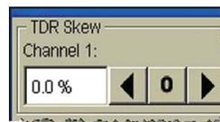
TDR skew regulates the time differential between the launches of TDR steps.
