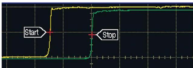
14. In the **Measure** table, locate the mean delta time value. This represents the added travel time (out and back) introduced by the additional cable length.
