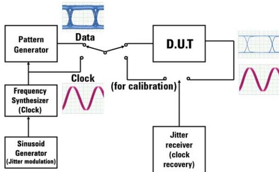
Figure 8: The test system is capable of four possible combinations of clock or data at the input or output of the test device
