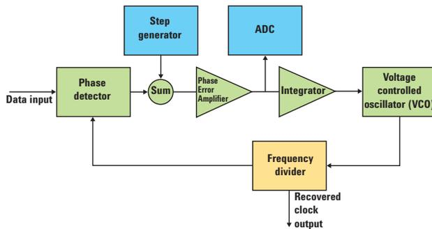
**Figure 17. Block diagram of the 83496B**
