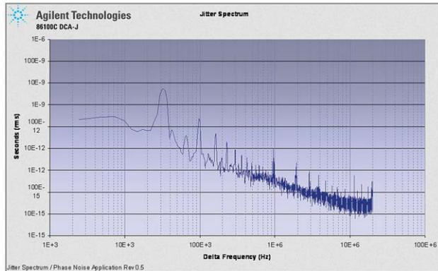
**Figure 13. Jitter spectrum of the PCI Express reference clock**
