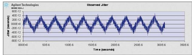
**Figure 14. Jitter of a clock signal having passed through virtual PLL's and transport delay**
