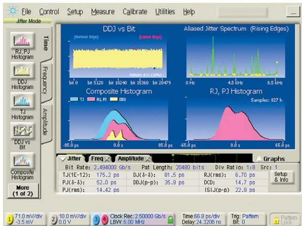
Figure 10. Jitter histograms and components for a 2.5 Gb/s PCI Express data signal using 86100C jitter mode
