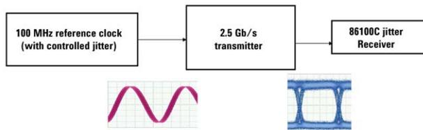
Figure 6: PLL/jitter transfer test system block diagram
