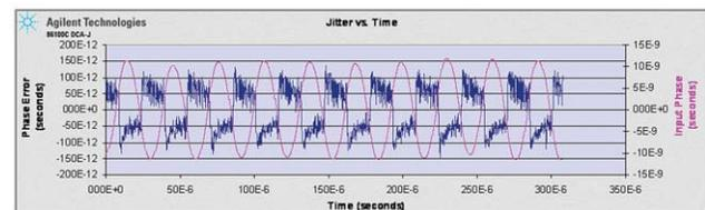
**Figure 16. Input phase and phase error**
