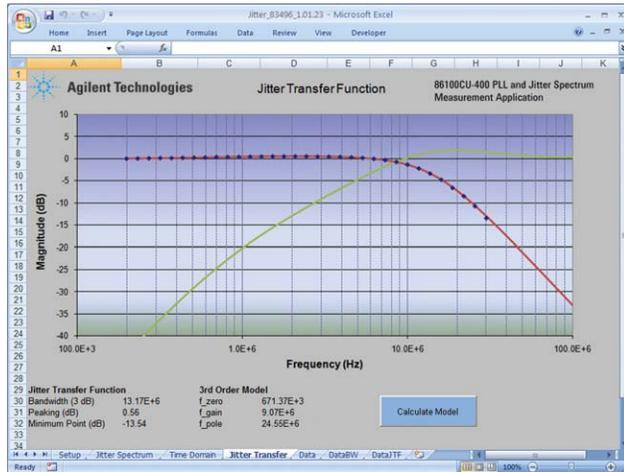
Figure 7: Jitter transfer/PLL bandwidth result for a PCI-Express transmitter
