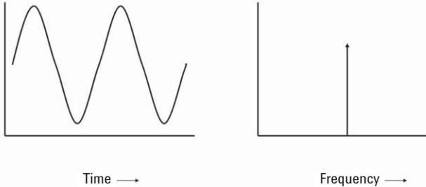
**Figure 2. Time and frequency representations of a simple sinusoid**
