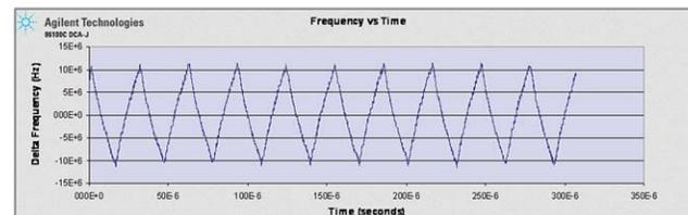
Figure 12. Delta frequency versus time for a PCI Express data signal
