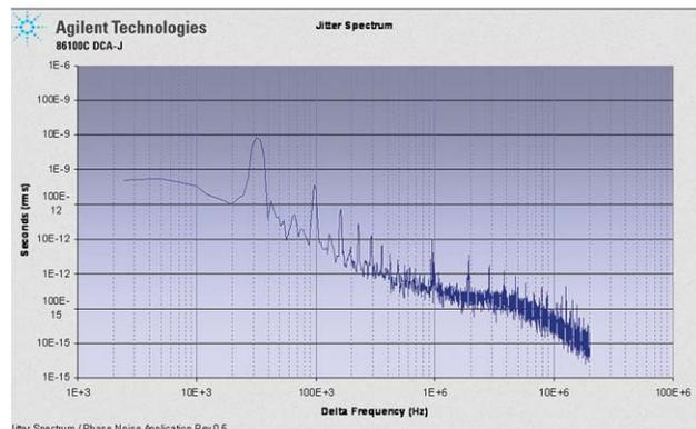
Figure 11. Spectrally resolved jitter of a PCI-Express data signal
