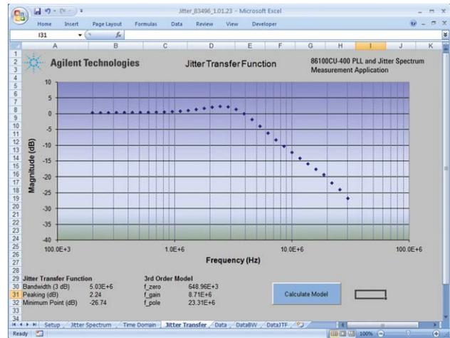
Figure 9: Jitter transfer/PLL bandwidth result for a 5 Gb/s clock recovery circuit
