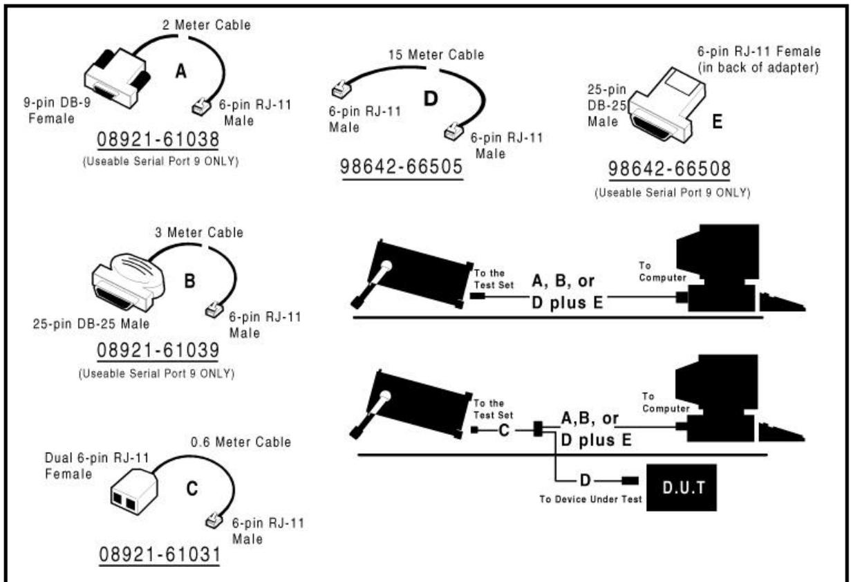
**Figure 2-2. Connecting the Test Set Serial Port to a PC or Terminal**
