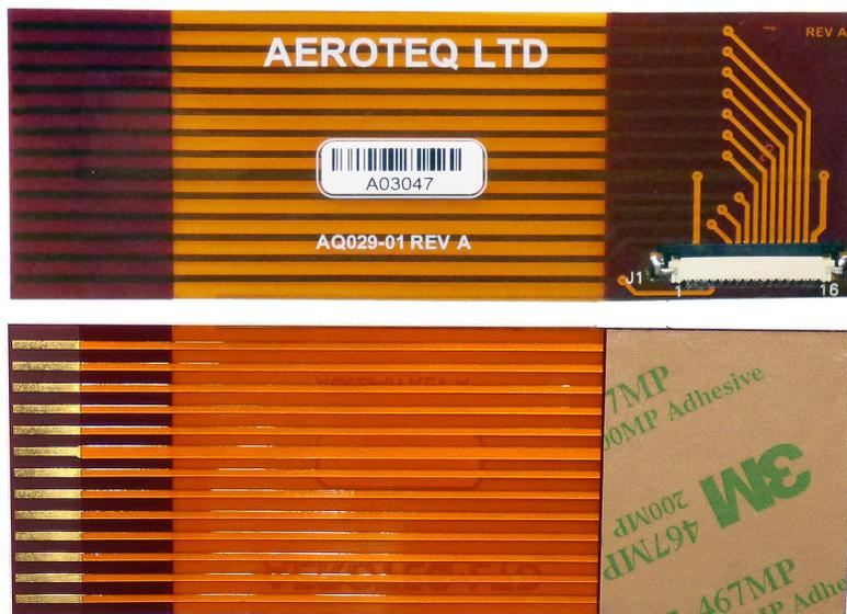
Figure 20 A custom designed flexprint adapter cable.
