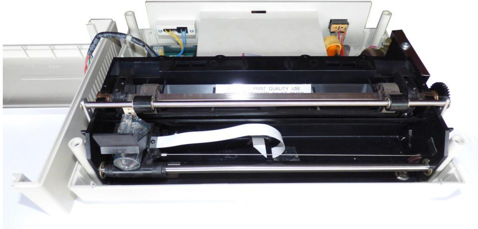
**Figure 18** The Flexprint cable can be pre-bent to keep it in the desired shape. Note the plastic clip clamping its end to the chassis bottom. You can see a loop of the Flexprint adapter ribbon cable peeking out over the front edge of the battery box – it could have been shorter. On the other hand this loop allows placing the ZIF connector into the space between chassis and battery box without interference or risk of short circuits.
