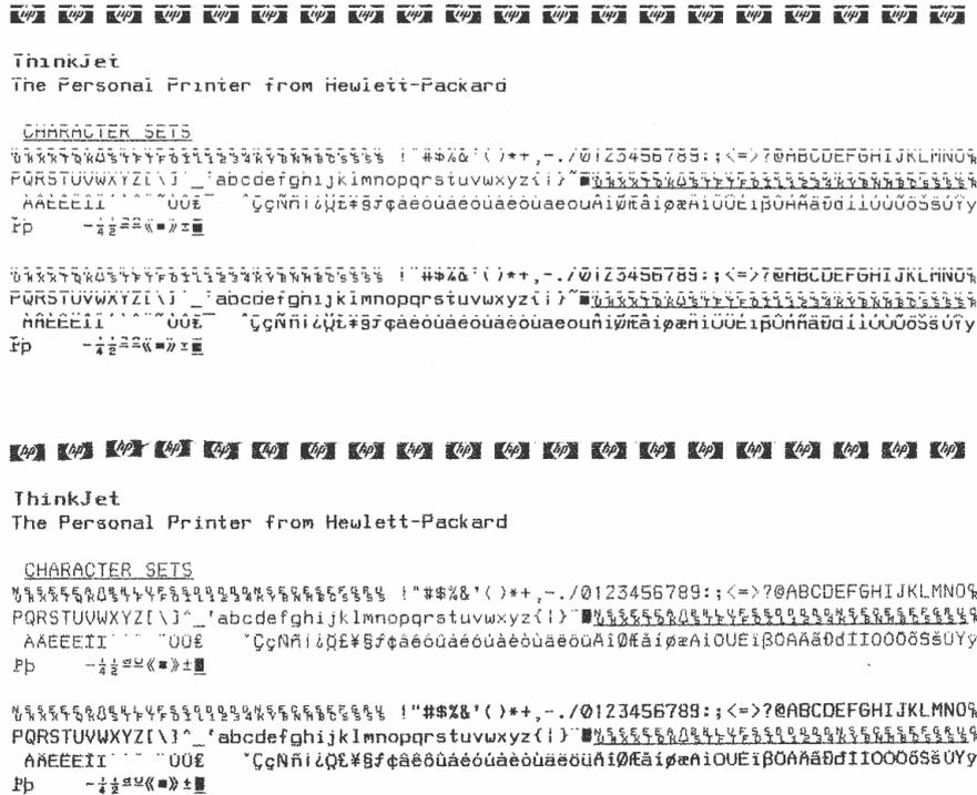
Figure 21 Test printouts. Top: original cable with two dot rows missing. Bottom: repaired ThinkJet with all dots printing. Wavy regions are not a fault of the printer but mine due to sloppy single sheet paper loading.
