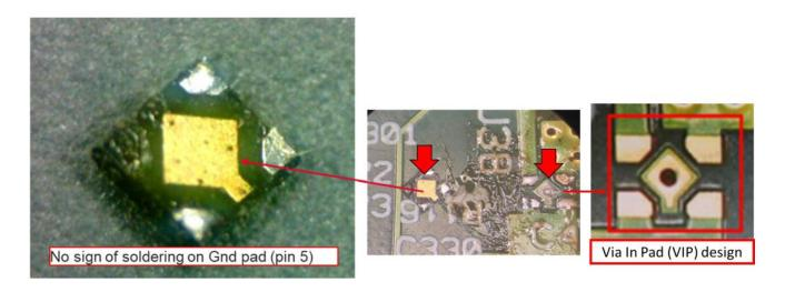
The improvements were made from Via in Pad (VIP) to Via in Pad Plated Over (VIPPO) as per below.
