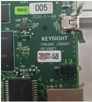
After PPMC board replace with 11713-63002 Programmed PPMC board, continue with instrument repair procedure.
