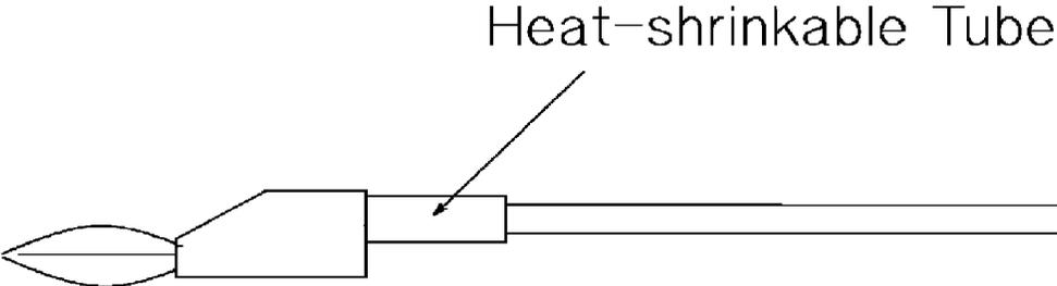
Figure 1. Improved Cable Assembly
