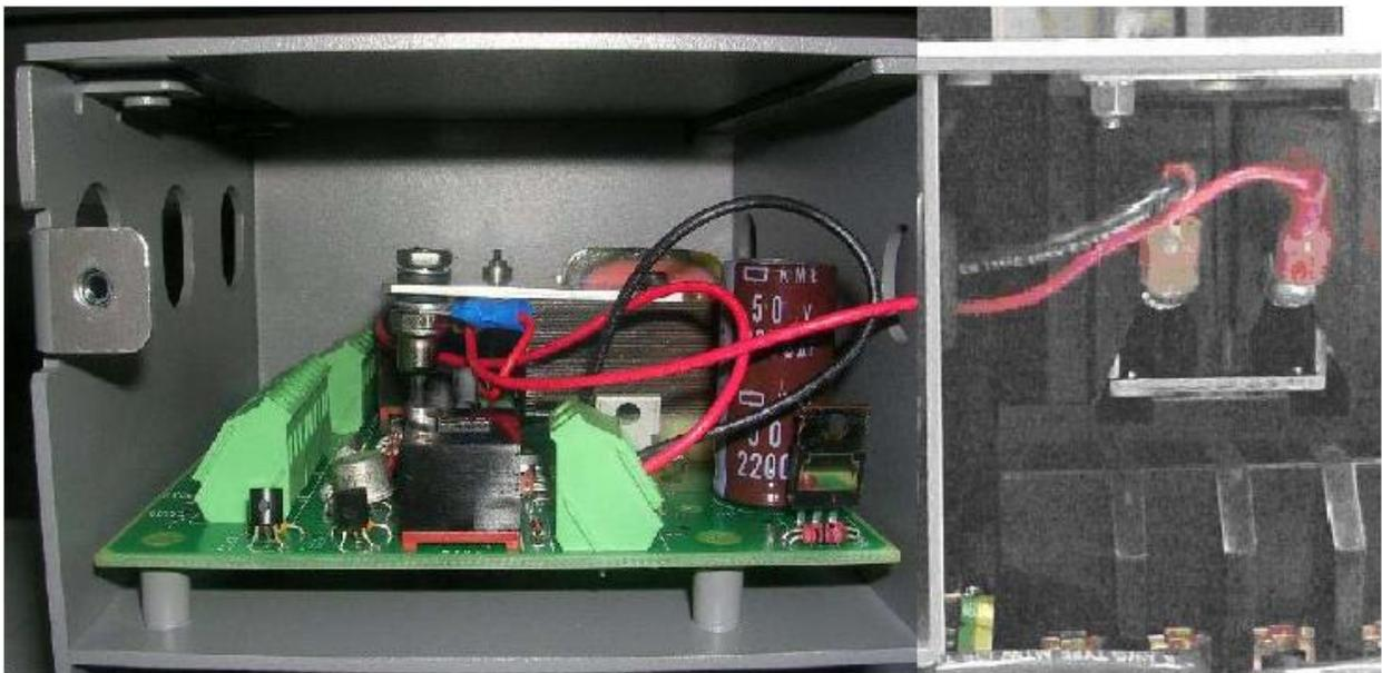
**Fig 15** (New Control board with voltage regulator)
