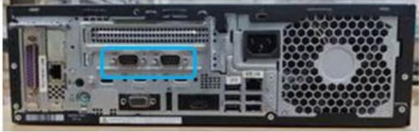
Figure 2a: Wrongly configured Serial ports
