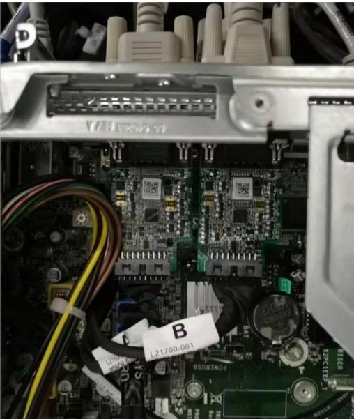
Figure 5: COM1 and COM2 are installed
