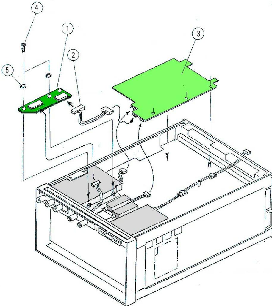
**Figure 1 Filter board replacement**
