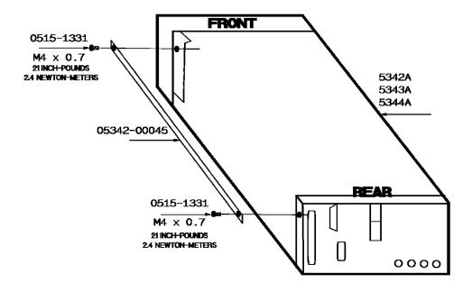
Figure 1. HP 5342A/43A/44A Orientation and Support Strut Installation
