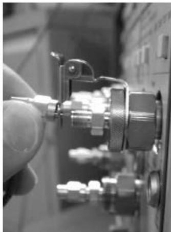
Figure 2. Shorting test cable.
