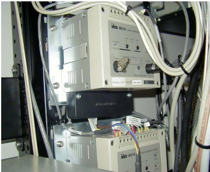
**Figure 6B: Laser supply with N7200-04125 cover installed on Series 3/5000**
