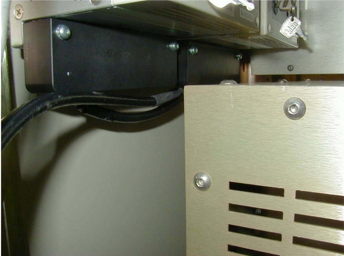
**Figure 2: Laser supplies with N7200-04125 covers installed**
