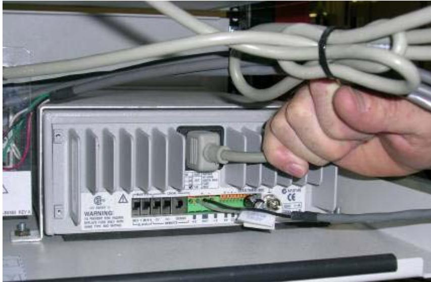
5. If the “AC Module” pulls out of instrument you will need to replace the E3615A. If the “AC Module” remains in place skip to step 13.
