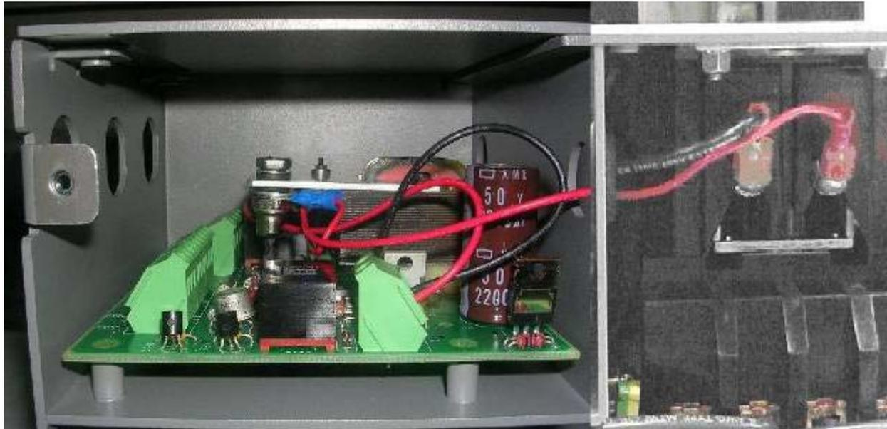
**Figure 15** (new Control Board with voltage regulator)
