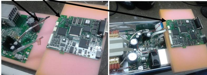
Remove the connector P/N 1252-3695 (circuit reference) "J206" on the "A2" interface assembly. When removing "J206" care should be taken not to damage the "A2" printed circuit board material or the circuit board traces. "J206" has 4 holes remove the solder from these holes as shown. Do not apply too much heat or pressure this may cause damage to the PCA
