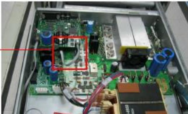
17. Connect cable (5080-2209) to F101 GPIB from the transformer.
