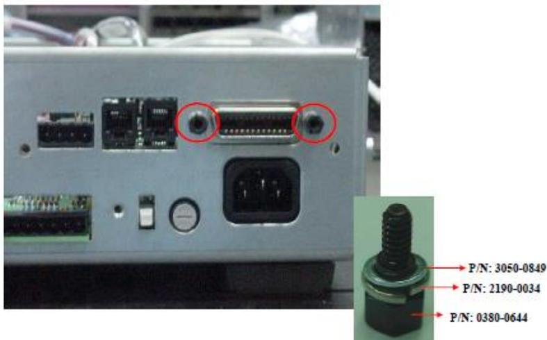
14. Secure with 2 screws as shown.
