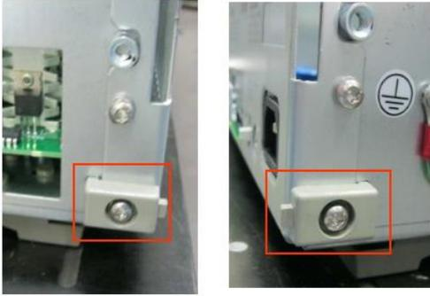
3. Remove the screw at each side of the chassis.
