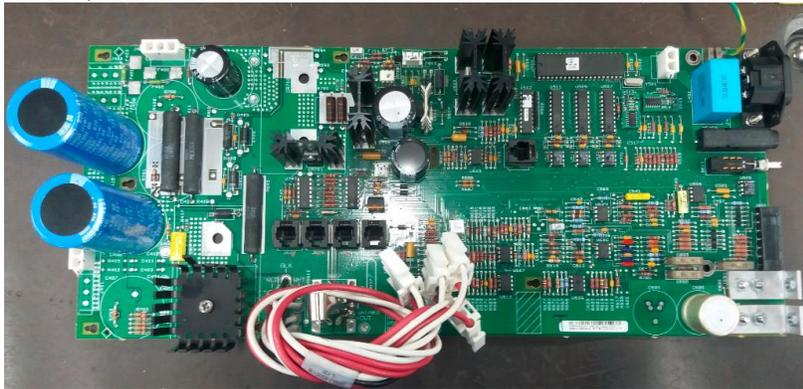
11. Lodge the PCA into the 6 key pin, then slide to lock it to the chassis.
