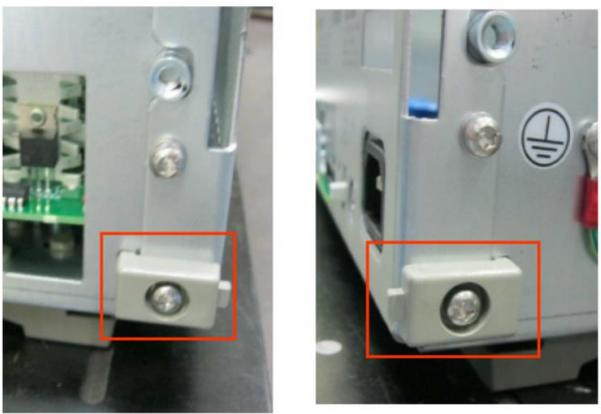
22. Mount the handle, front cap and back cap to both sides of cover with 2 screws as shown in the
