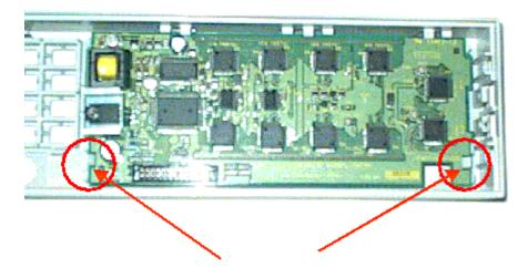
Carefully press aside these plastic clips while installing or removing the display!
