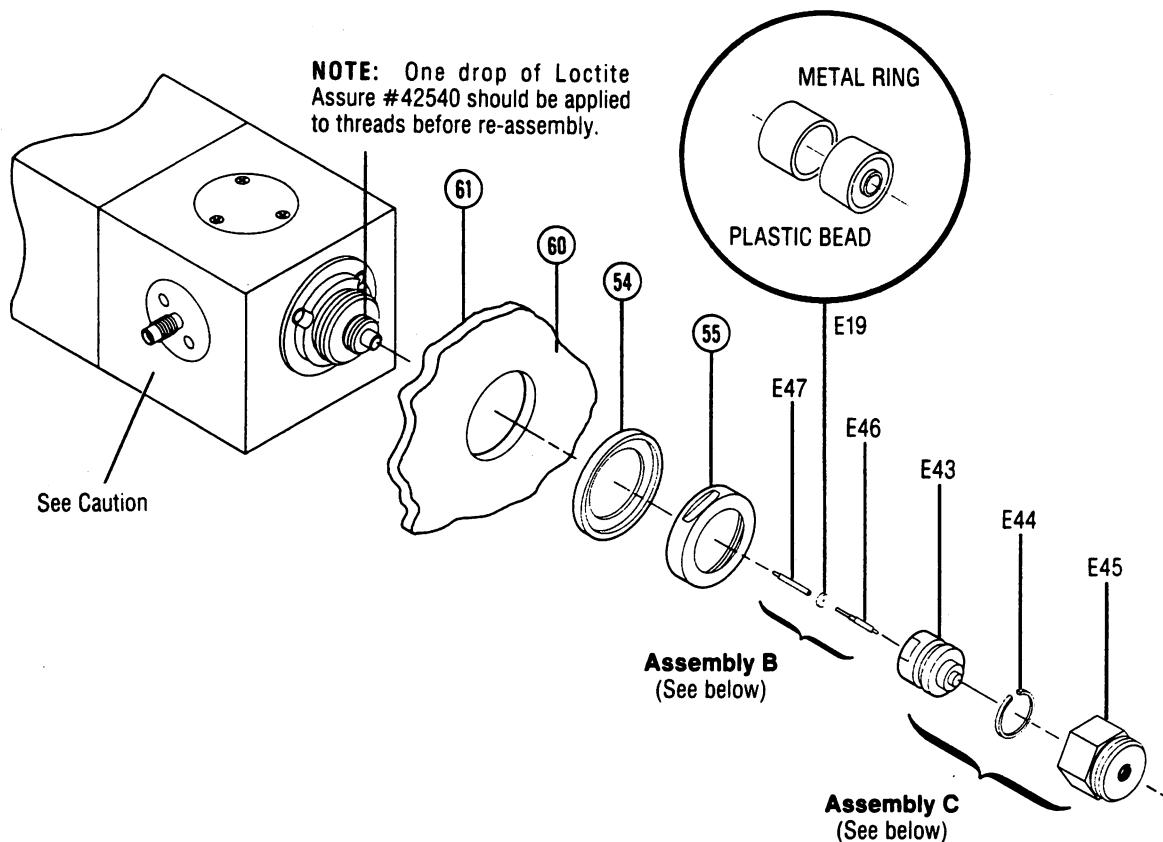
**ASSEMBLY B:** These 3 parts are locked together. Replace all three at the same time by ordering Test Bead Assembly HP P/N 5061-5355. Don't confuse the metal ring with a shim.
