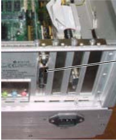
A11GPIB Board Assembly inserted in the A4PCI 1 Slot with previous revision of the A4 Motherboard
