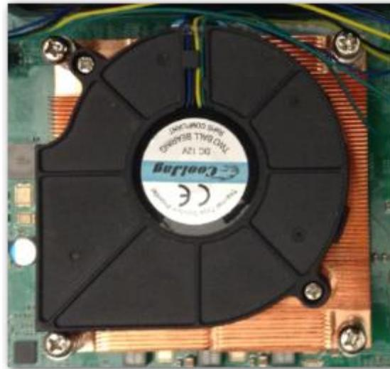
The mass of the heatsink requires additional mounting points only found on the N1000-00045 chassis plus a special mounting plate.
