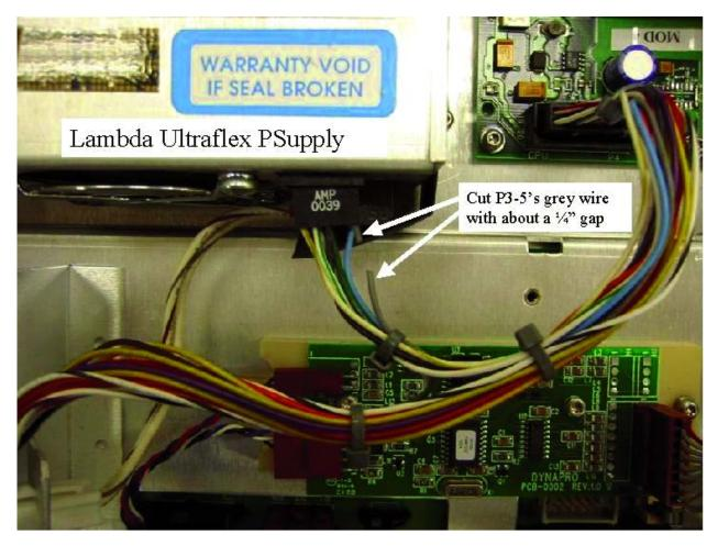
**Note:** Both the PFW and Fan/Thermal outputs are open collector, and wire-or'ed together on the Power Supply Distribution board (A1A2, 86130-60001). If the GREY wire (Fan/Thermal) is cut and the proper PLD code is in place, the 86130A will only respond to valid power fail warnings (PFW's – refer to SN86130A-06A).
