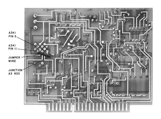
Figure 1. A3K1 PIN 11 to PIN 5 Jumper Wire on Circuit Side of A3 Reciprocal Amplifier Board
