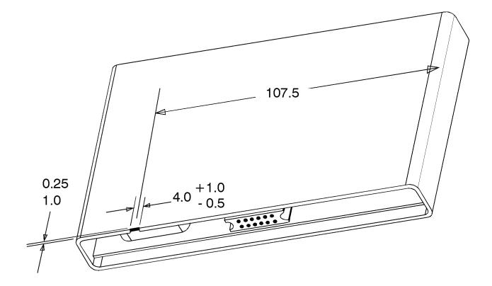
Part Number 08720-60156 2nd Converter Add Notch As Shown. Exact Form Not Required. Semi-Circle or "V" Notch Are Acceptable. All Dimensions Are In Millimeters.
