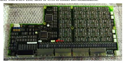
4. Board Installation – Return the PCA back into the module housing by reversing the removal steps. Remember to plug the DC power cable to the PCA prior to installing the top cover.
