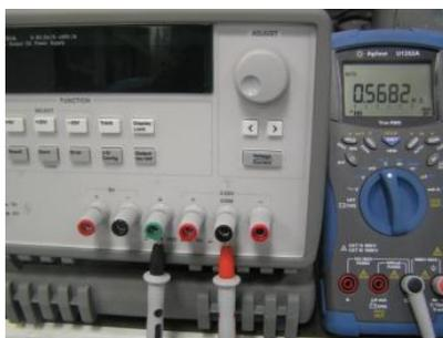
$\pm 25\text{V}$  output power line's common terminal to ground terminal
