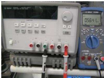
$-25\text{V}$  output power line to ground terminal
