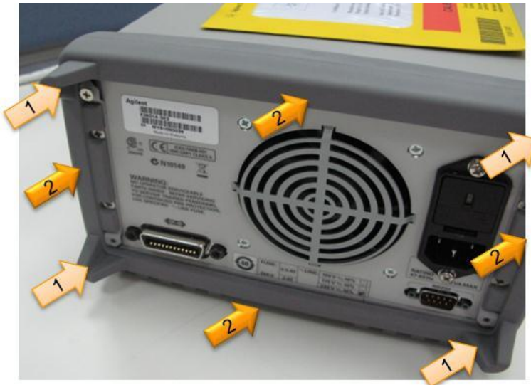
Figure 2: Proper fitting method for instrument rear bumper
