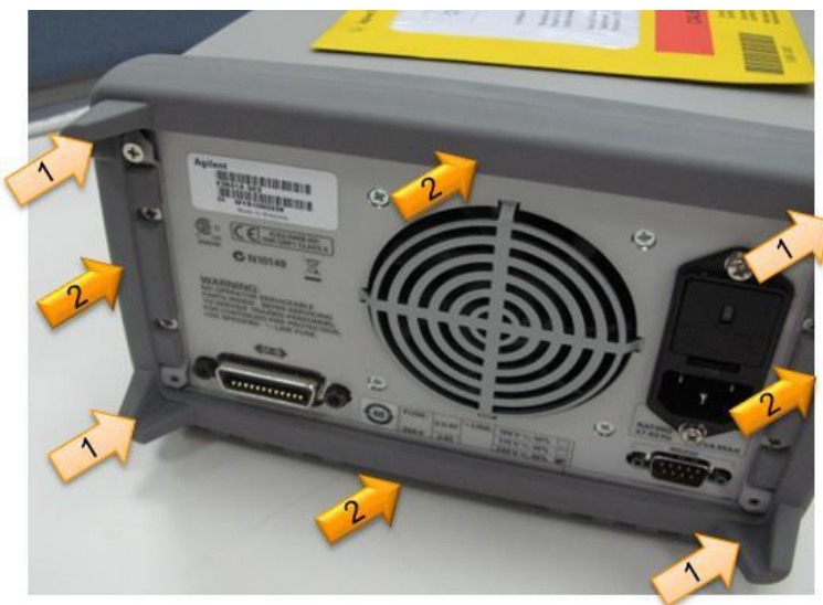
Figure 2: Proper fitting method for instrument rear bumper
