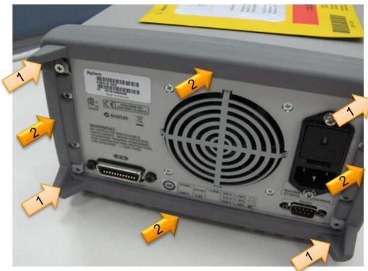
Figure 2: Proper fitting method for instrument rear bumper
