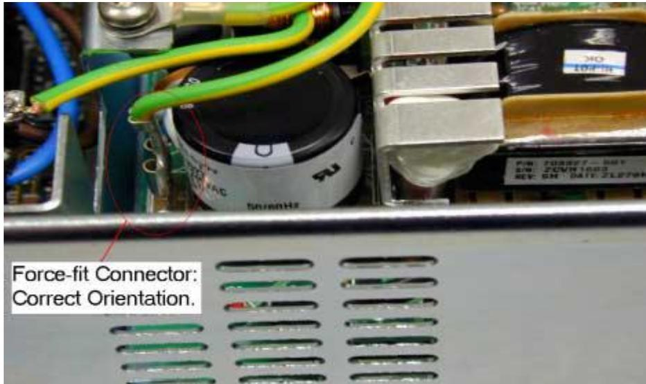
Figure 3: Correct orientation of force-fit connector.
