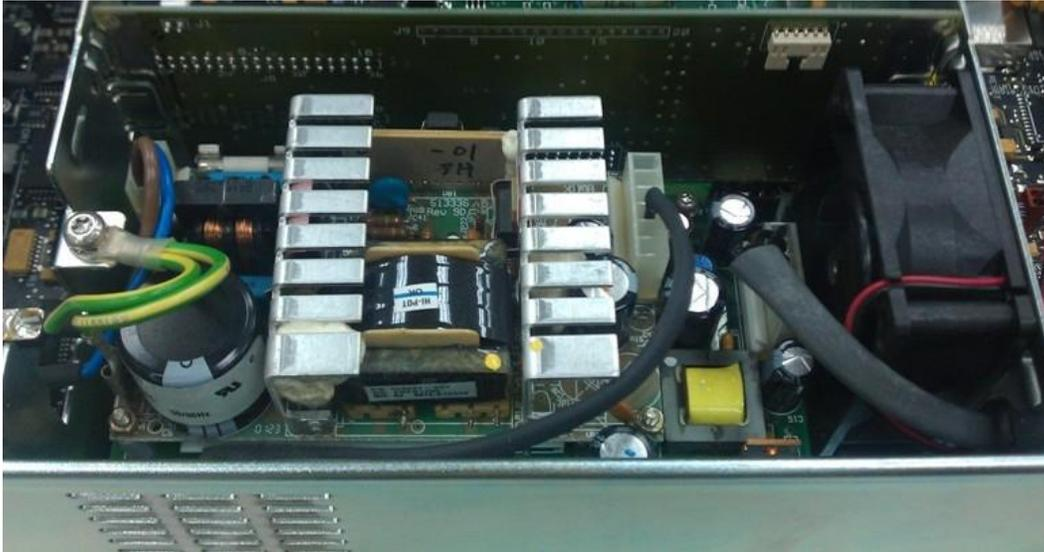
Figure 1: Interior Layout of Power Supply Unit, P/N: 0950-3681
