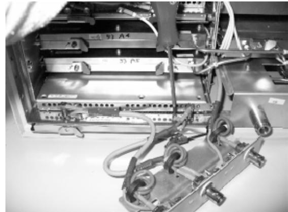
Figure 6 Install the A2 board back in the slot and put connectors back on the board
