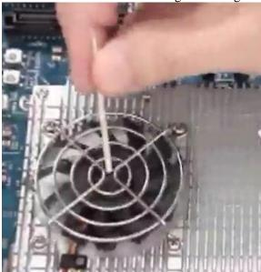
2. If CPU fan rotates, then the cause of the trouble is [dropped off rotor]
