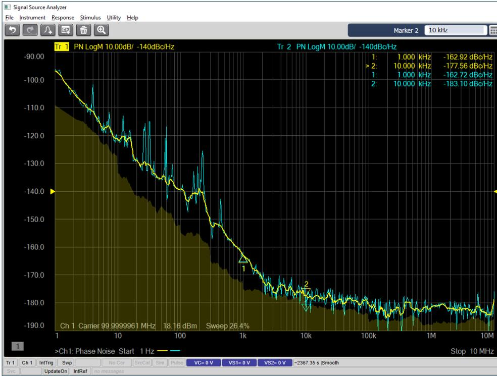
Fig 2. Measurement of DUT after replacing DDS modules
