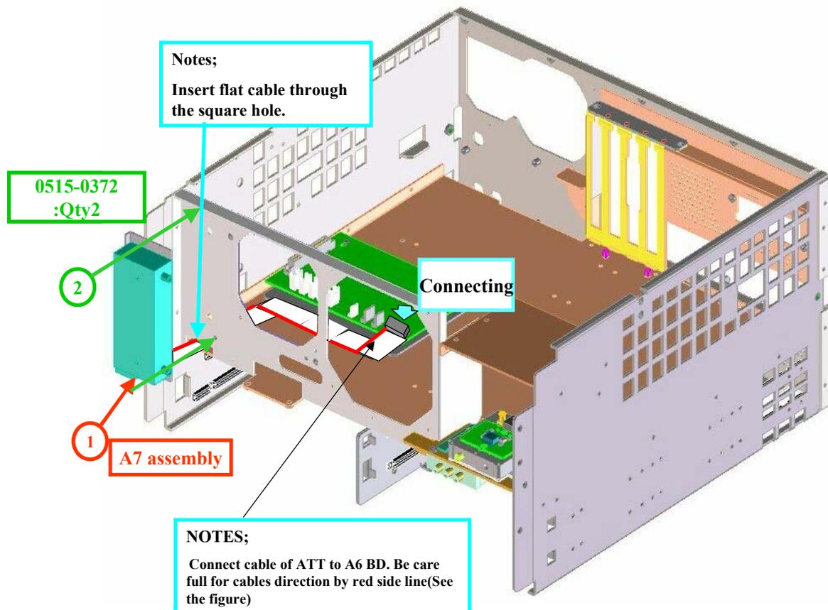
**Figure 3 Install A7 attenuator assembly (for option 213)**
