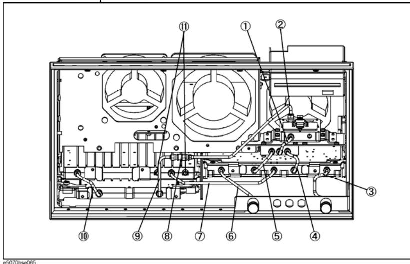
**Figure 1 Front View (Semi-rigid Cables Opt. 213 before modification)**
