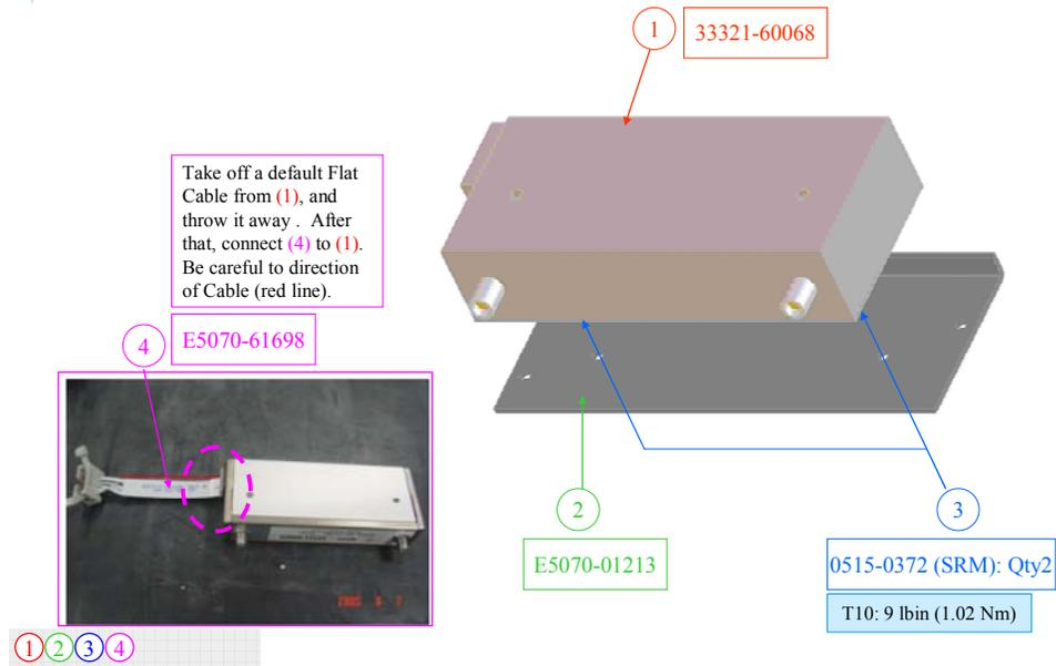
**Figure 2 Make A7 attenuator assembly (for option 213)**
