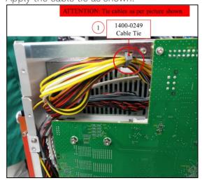
3. Apply the cable tie to the LVDS cable assembly. Push the cables downward. Note: DO NOT tie the USB cable.
