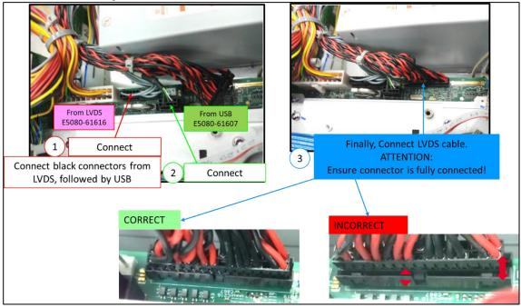
5. Ensure the cables are fully connected and routed as shown.
