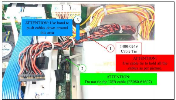
4. Connect the USB cable. Finally, connect the LVDS cable to the motherboard connector. Ensure that it is fully connected.
