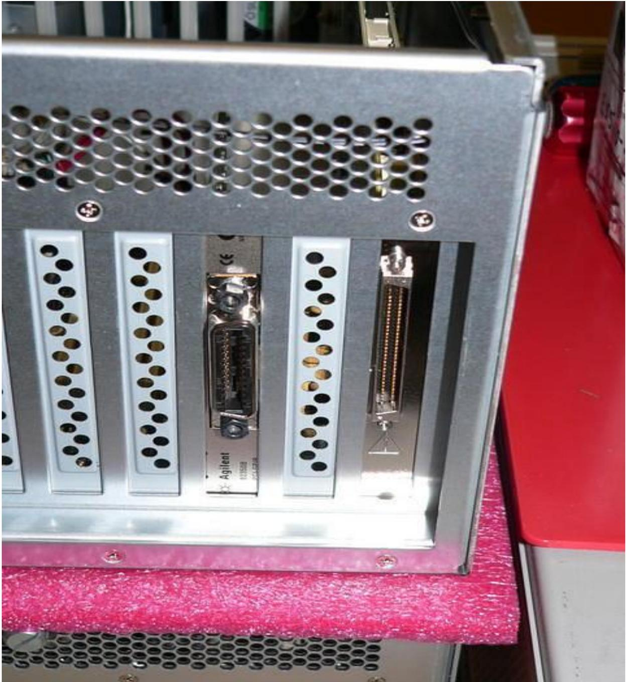
2. Shut down the computer and unplug the power cable. At a safe ESD work area, remove the cover from the Kontron PC by loosening the thumb screws and sliding the cover back.
